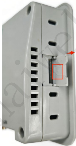
Figure29 Installation of 4-inch HMI with 4G Card
