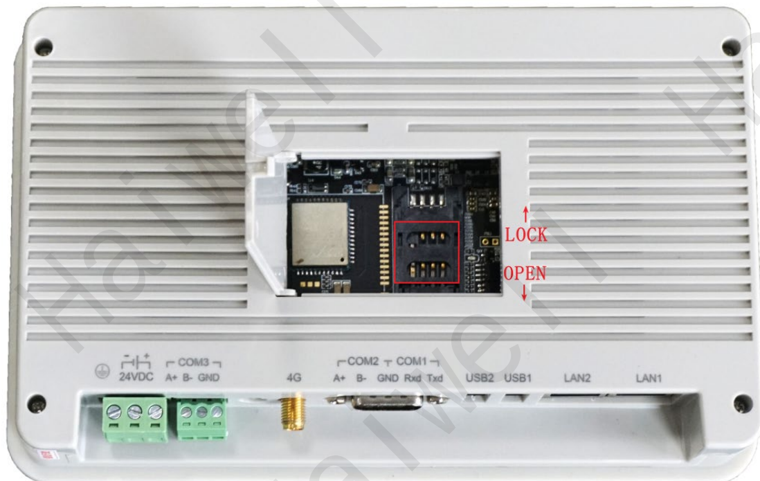
Figure25 HMI Installation of 4G Card
